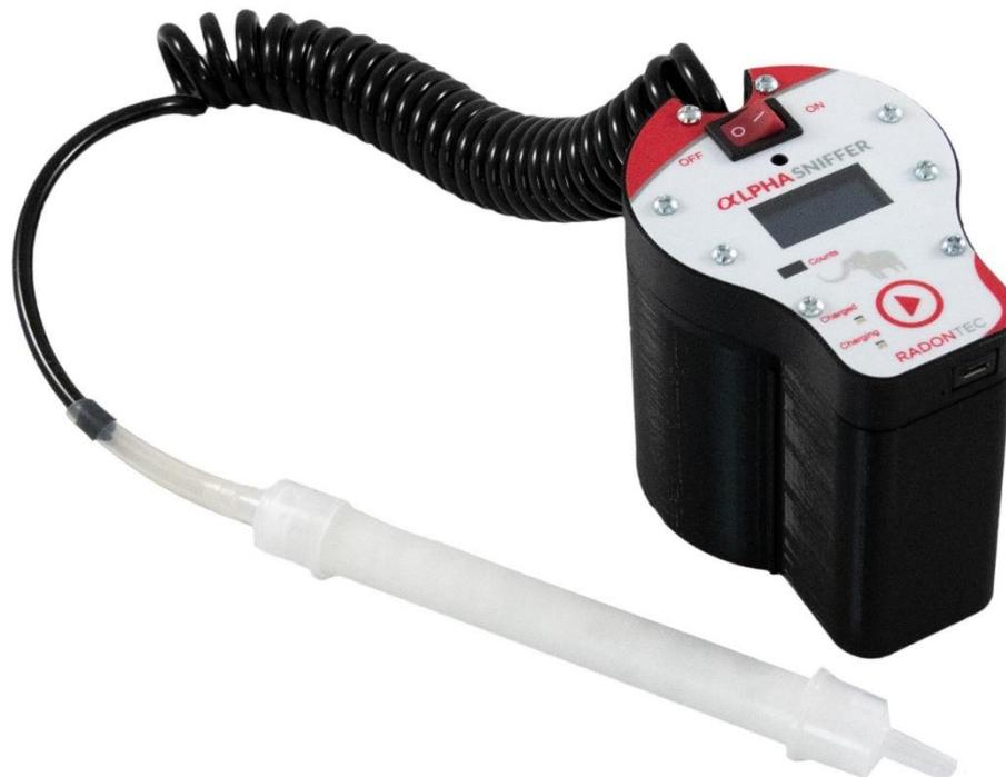
As radon decays inside the cell, the alpha particle emitted hits the wall of the cell, which is coated with scintillation powder, and emits a flash of light. The photomultiplier converts the light into an electronic pulse, which is then counted.
